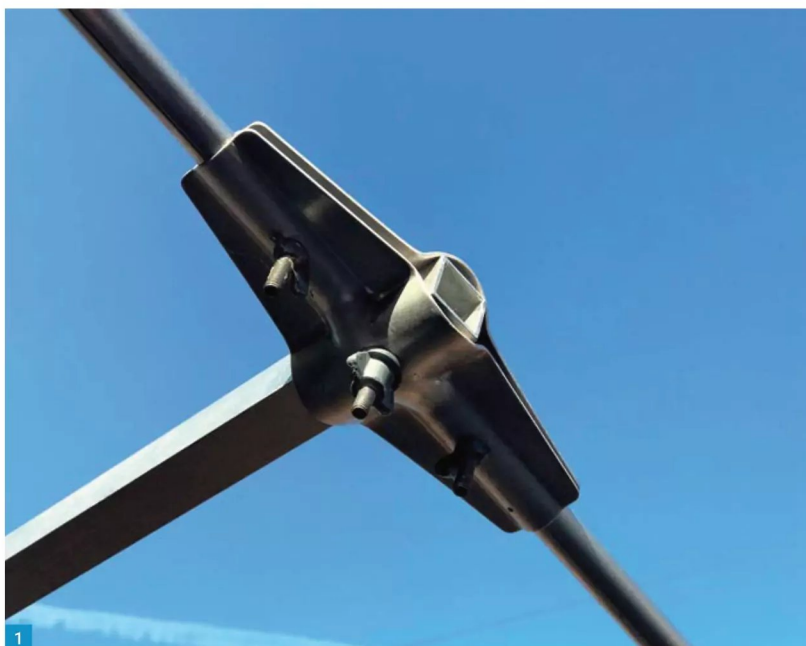
Fig. 1: The parts of the parasitic reflector are electrically connected as one solid element. Fig. 2: A ferrite collar is one option for a choke balun near the feedpoint.
