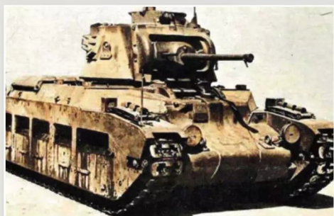
◀ Matilda II Mk IIA*: The standard version featured the Besa 7.92mm MG and the more powerful 94hp twin Leyland diesel engines
