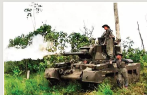
◀ Matilda II Mk IIA*: The standard version featured the Besa 7.92mm MG and the more powerful 94hp twin Leyland diesel engines
