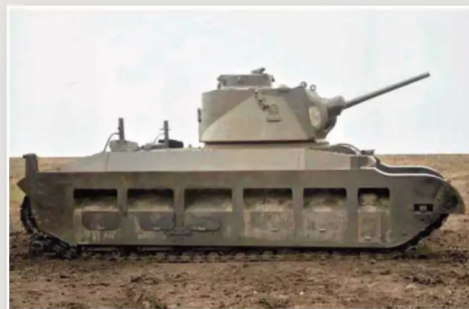
◀ A12E1 Matilda II Mk I: This A12 prototype featured six mud chutes twin AEC 87bhp engines and a Vickers heavy MG
