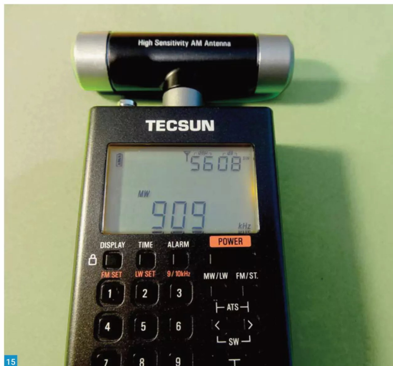
Fig. 15: The new Tecsun PL-368 has a separate, small, ferrite aerial for MW. (Nevada/Tecsun)
