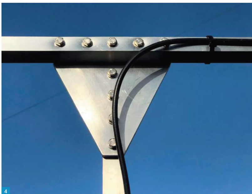
Fig. 3: The feed assembly adds 3cm to each leg of the driven element.
